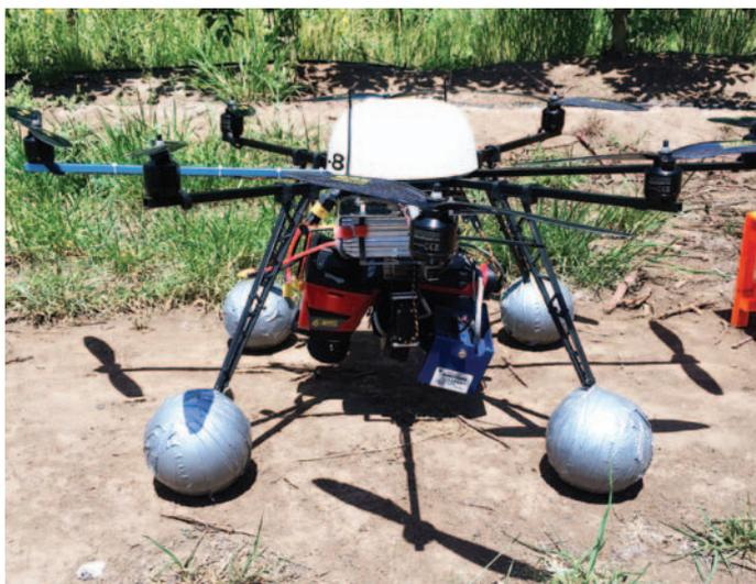
Eye in the sky: Octocopter from the VoF - Chile preparing for a measurement flight. This octocopter carries a thermal camera, a normal visible camera and a multispectral camera.
