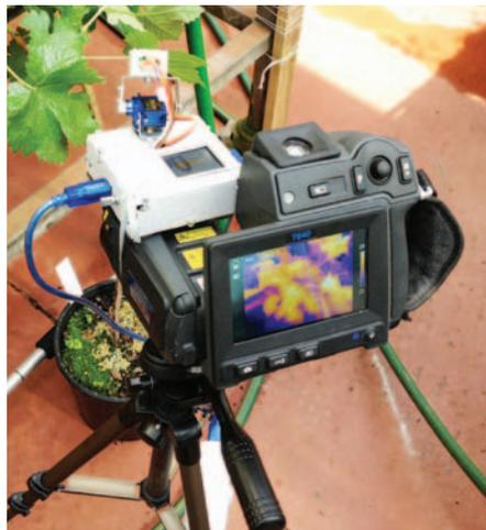
Say cheese: Infrared camera taking a thermal image from grapevines in the glasshouse. On top of the camera is an IR scanner with a 1 per cent cost compared to the thermal camera which is currently under testing by the VoF (Australia - Chile).
